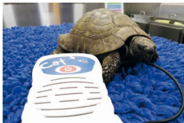
Figure 1. An 8 MHz Doppler probe, such as those used to measure feline blood pressure, can be used to check for a carotid pulse.
