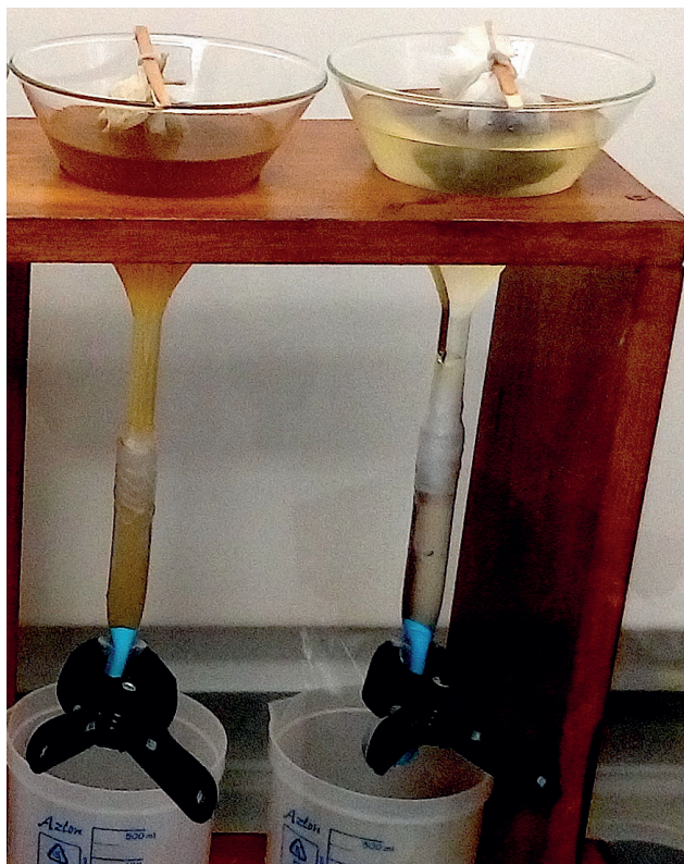
Figure 2. Baermann apparatus used for the isolation of lungworm larvae from the faeces of infected dogs.
