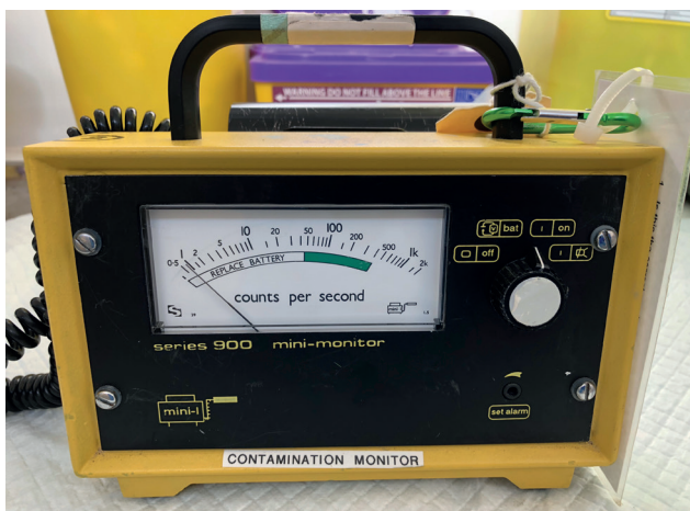
Figure 5. Hand-held Geiger counter used to measure radioactivity levels in patients and waste.
